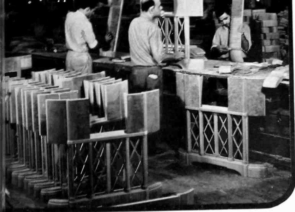
Preparation of front panels for cabinets. RCA Victor's wood-working machinery is spread over some 600,000 square feet of floor space
