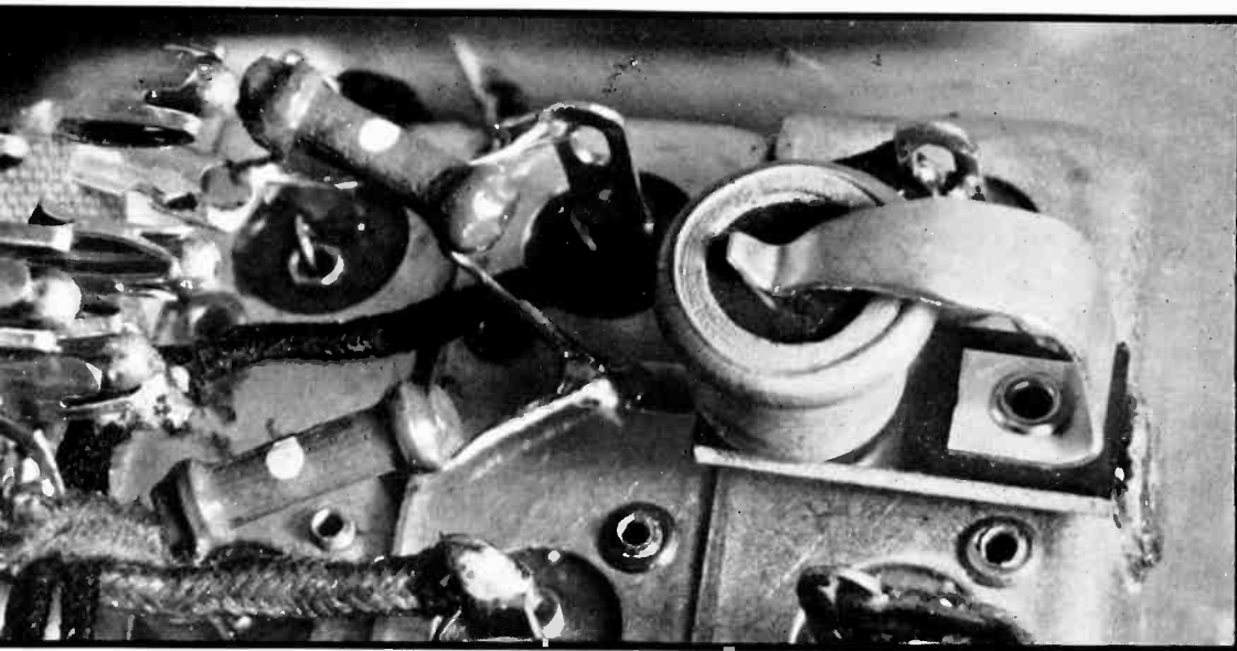
Close-up view of the grid-bias cell (twice actual size)
