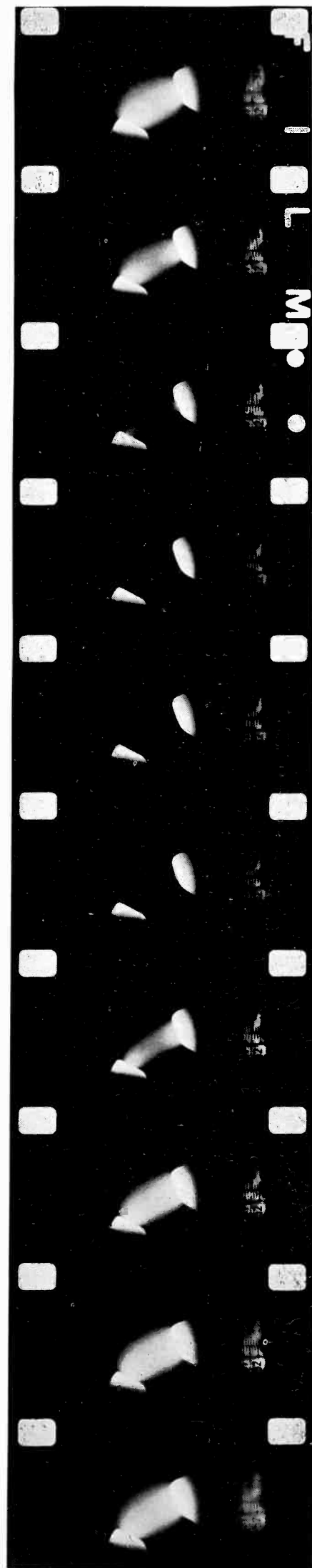
▶ Exposures taken at 1200 per second, of a carbon arc operating on 60-cycle current. One-half of a cycle is shown
