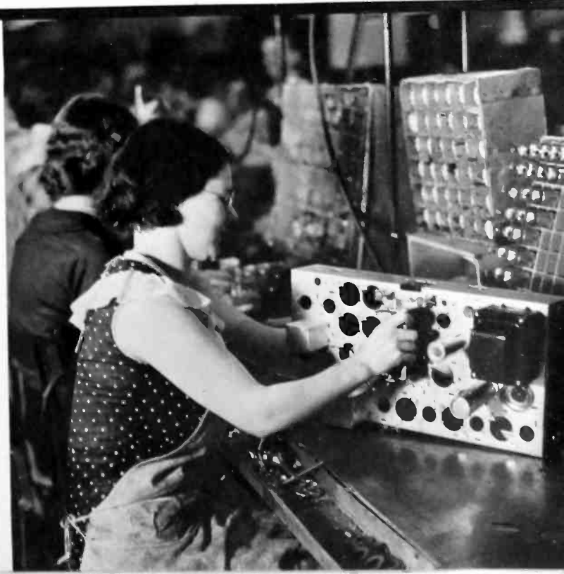
3 Another step along the feeder line. Here the major component parts, coils, condensers, transformers are added
