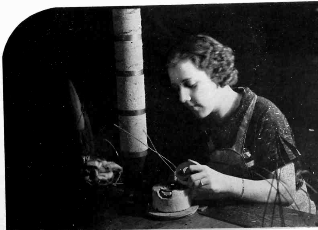
Joints of transformer coil leads dipped in silver solder insure per-
