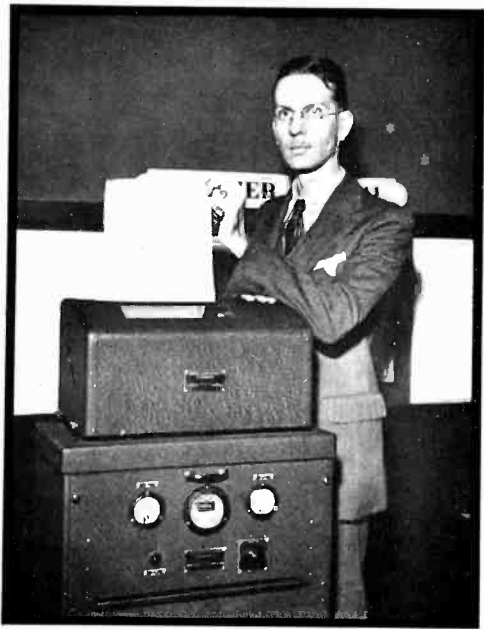
Apparatus to be used on passenger liners for receiving weather maps and newspapers by facsimile
