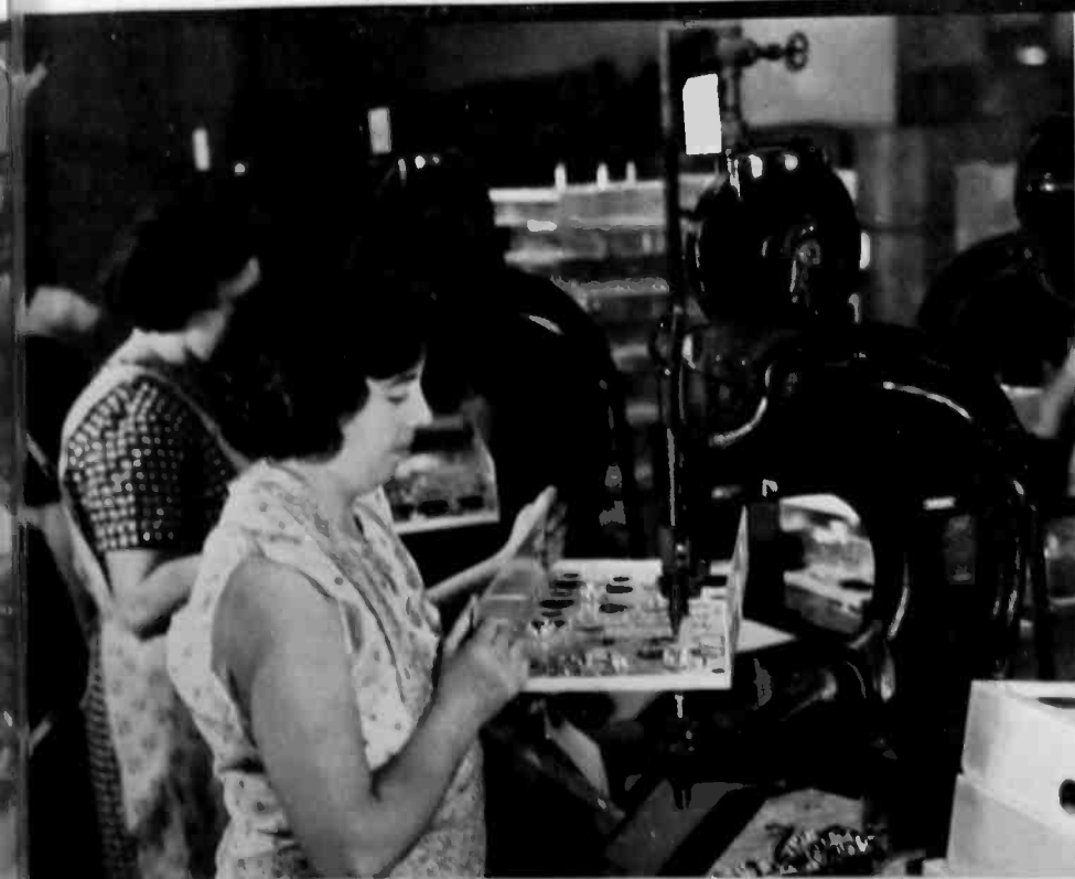
2 One operation on the feeder line. Riveting of sockets and miscellaneous components to the chassis proper
